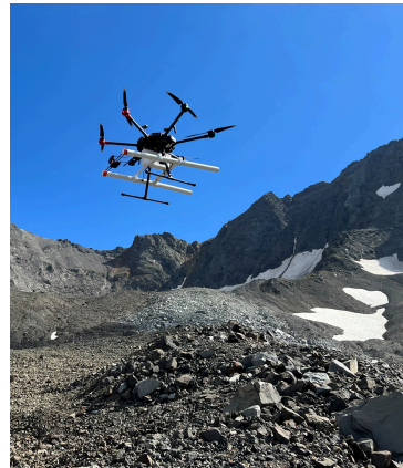
Figure 1: Drone GPR operations at Galena Creek, Wyoming, location marked with a red star in Fig. 3. The GPR MALA Geodrone 80 (white box) is mounted on the DJI M600 Pro drone. The length of the antennas is 1.04 m, with a separation of 0.5 m.
